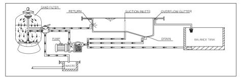
A suction is taken from the main drains on the bottom of the pool and the skimmers at the pool surface or balance tank and fed via separate pipework through the pump to the sand filter.
